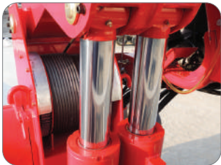
Heavy duty boom lifting cylinders
