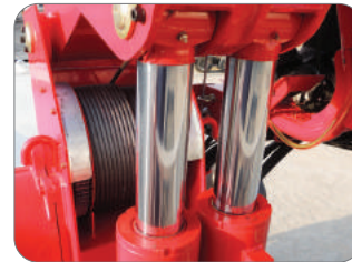
2 Derrick Cylinders Adjusted
